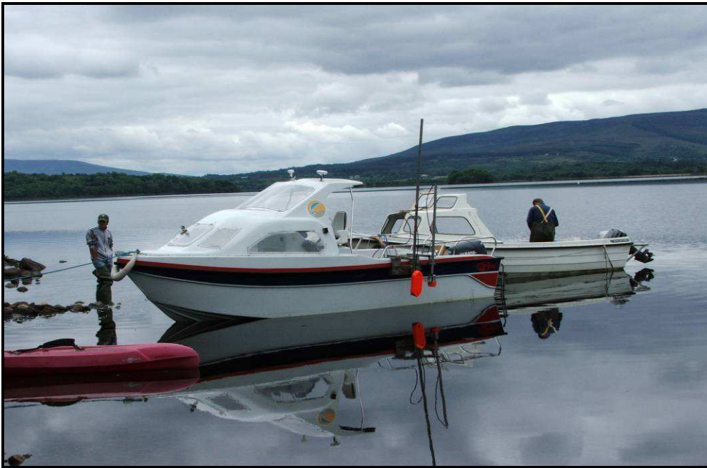
Plate 1.3: Hydroacoustic boat with two transducers (horizontal and vertical) mounted on the port side
